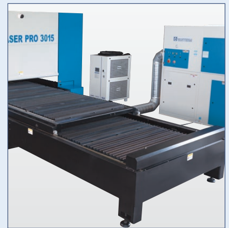
Automatic changer table system allows loading and unloading of table during the cutting process
