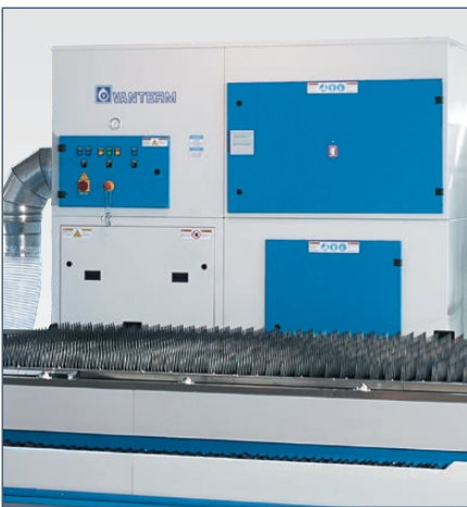
Machine comes standard with dust collector and filtration unit which protects the operator and the environment against the noxious emissions from cutting operations
