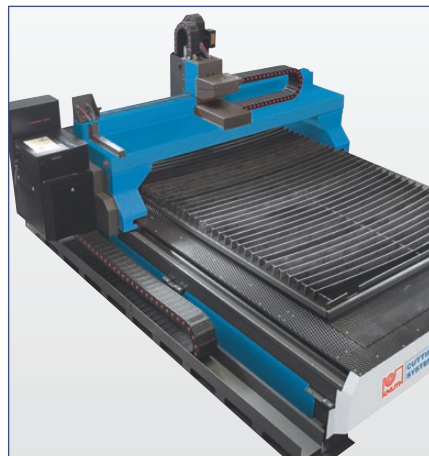
No thermal or mechanical influences on the guiding machine due to separate installation
