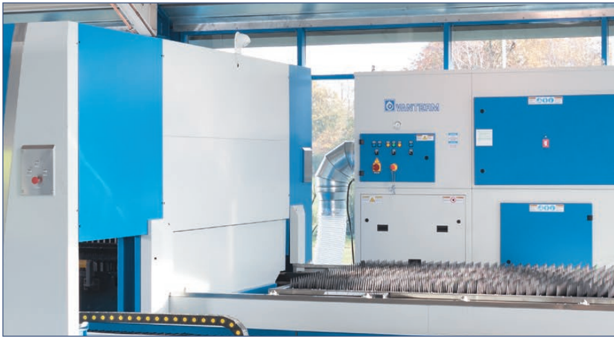
Filtered exhaust system with dust separator and a filtration unit
