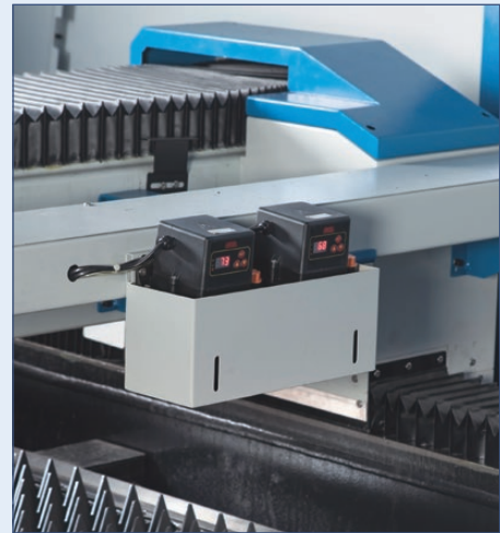
Central lubrication system: minimizes maintenance, increases reliability
