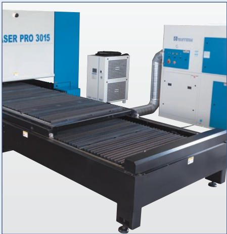
Automatic changer table system allows loading and unloading of table during the cutting process
