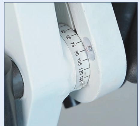
An angular stop ensures that every workpiece is bent with the same settings
