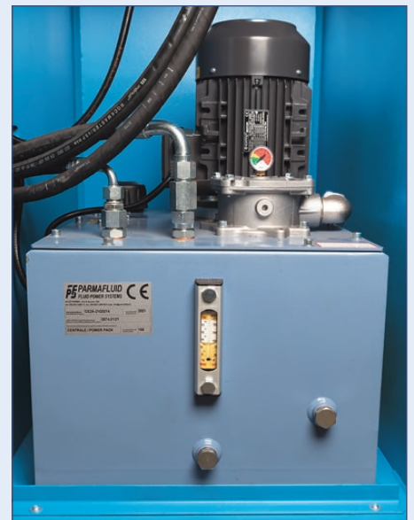
Space saving hydraulic system located accessibly inside the frame
