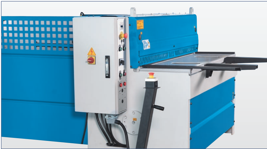
Back gauge is protected via sturdy enclosure and light curtain
