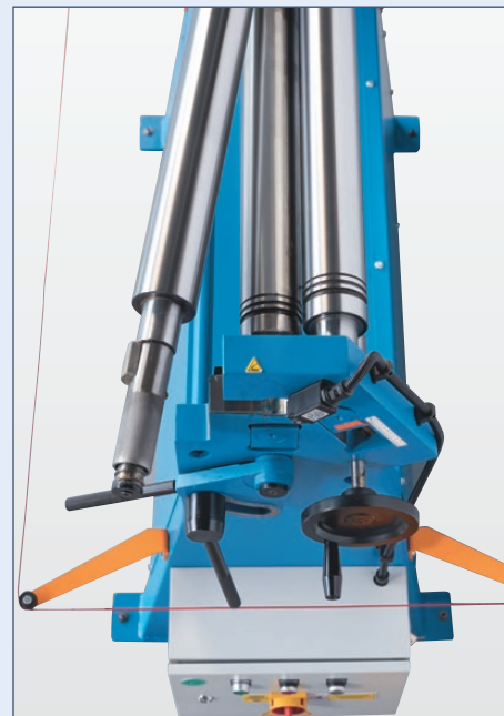
The upper roller swivels outward for easy removal of tube-shaped bent workpieces
