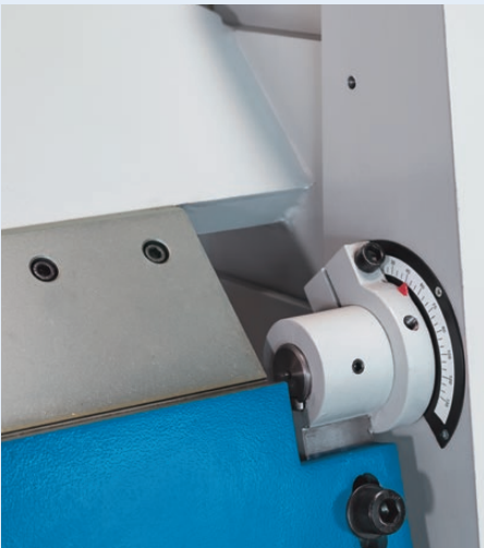
Exact bending angle across the entire work length
