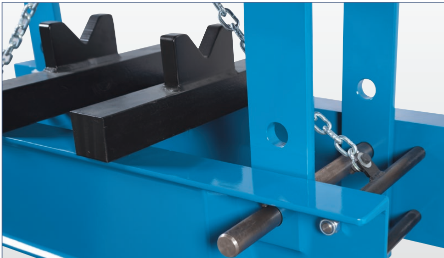
Standard v-blocks are very versatile and can be used for a variety of press work tasks
