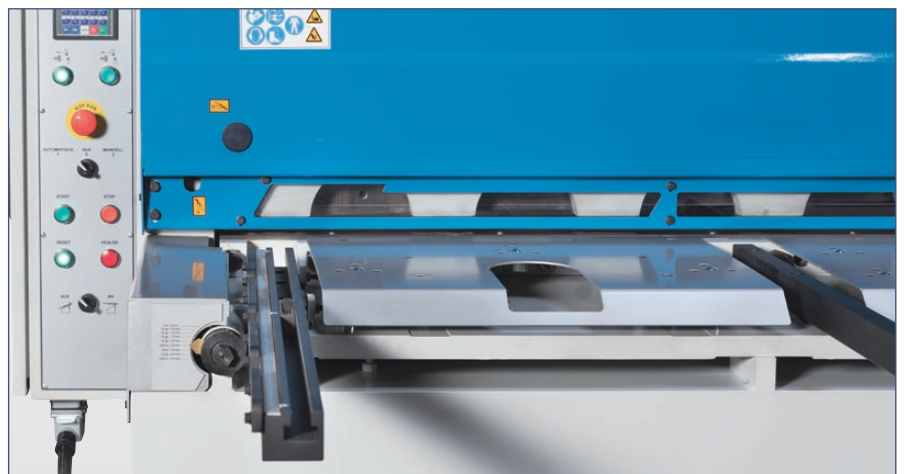
Lateral stop with scale and manually adjustable kerf setting
