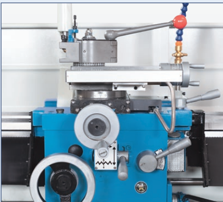
Support with enclosed oil-bath for low maintenance
