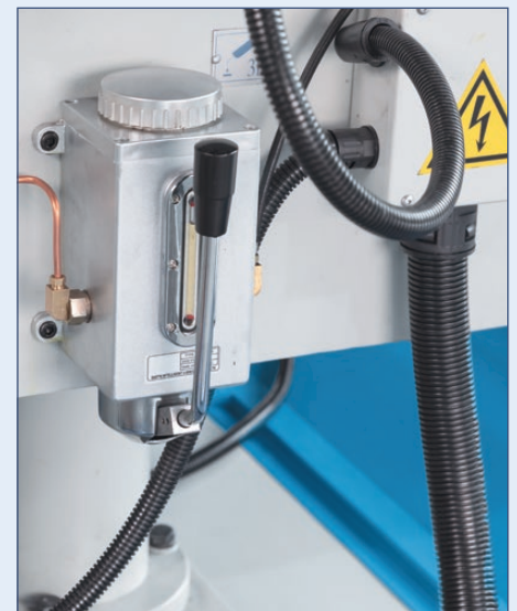
Central lubrication facilitates machine maintenance.
