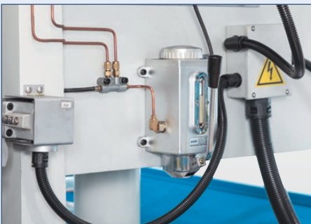
Manual central lubrication reduces maintenance and extends the machine life
