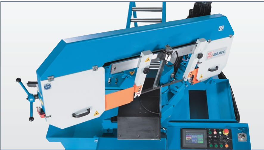
The saw frame swivels up to 45° to either side
