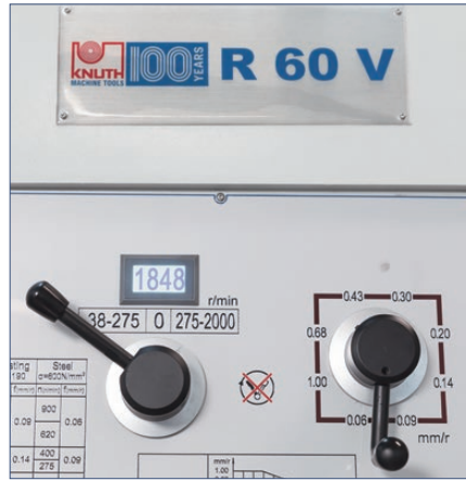
Infinitely variable spindle speed and easy to read digital display
