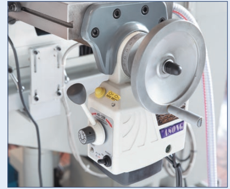
Automatic feed and rapid feed are infinitely variable and provided with adjustable back gauges
