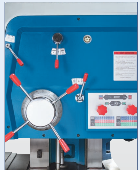
Headstock and feed gears are equipped with an overload clutch
