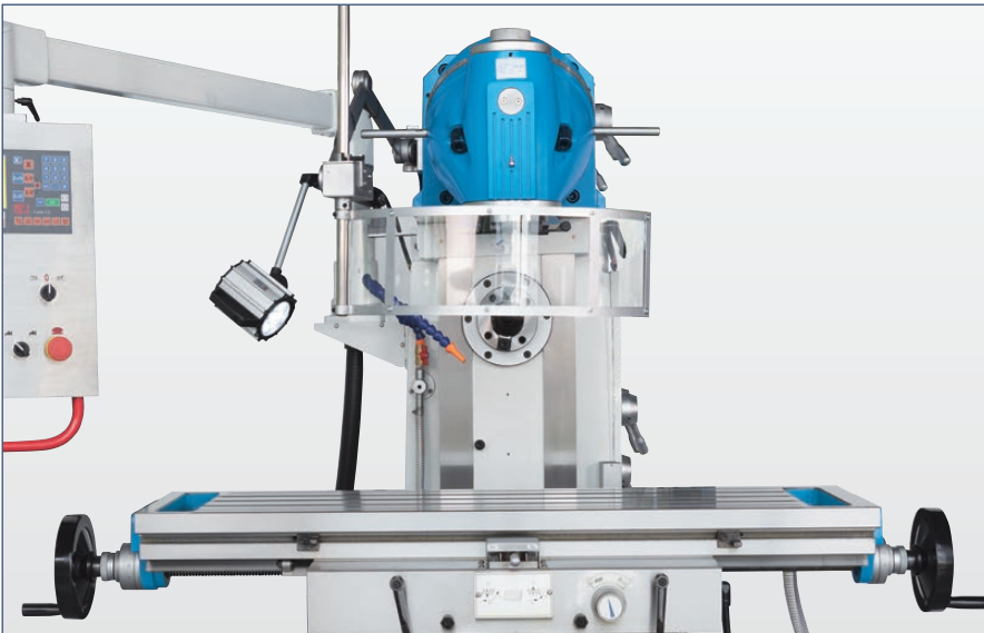
Large working area of 1325 x 360 mm and up to 500 kg table load
