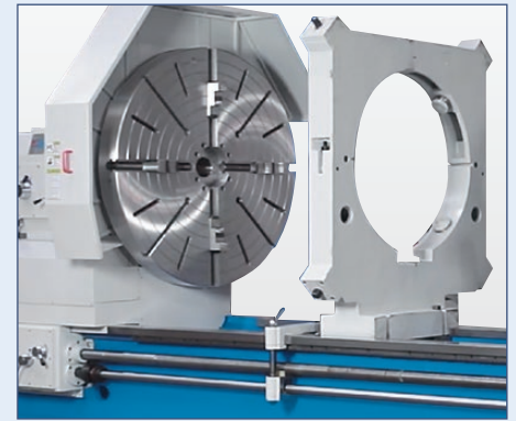
Rests are indispensable when machining long workpieces
