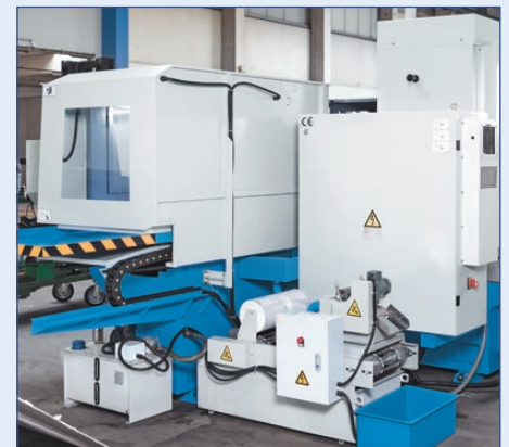
On the moving column design, the grinder table travels directly on the wide machine bed
