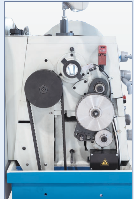
Change gears provide for a wide range of thread leads and feeds
