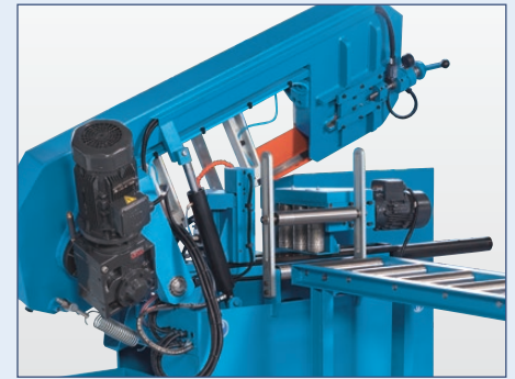
A motor with infinitely variable speeds transmits power via a continuous-operation idler gear to the machine drive wheel
