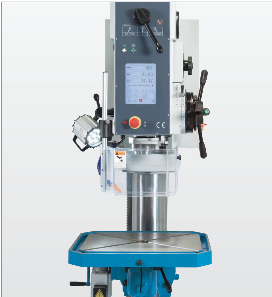
The wide speed range is controlled in two gear steps via inverter
