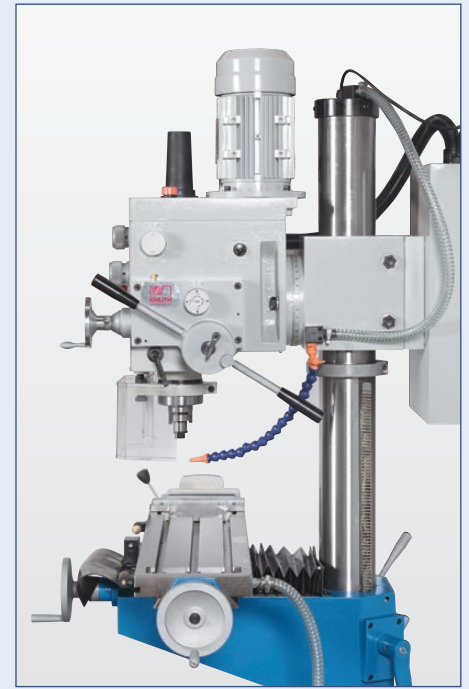
Automatic quill feed with 3-step gears
