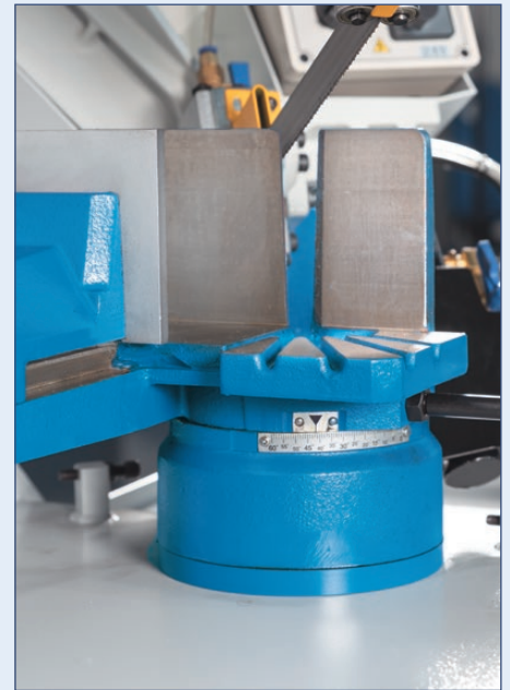
The scale ensures exact angle positioning
