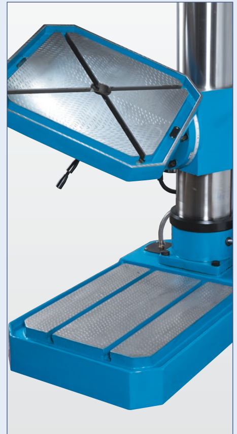
The large work table with diagonal chip flutes can be rotated and swiveled
