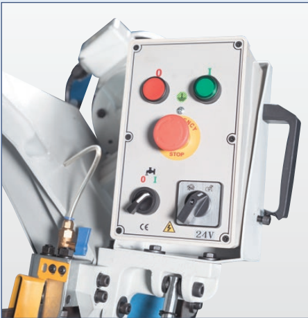
All functions are accessible on a compact control panel
