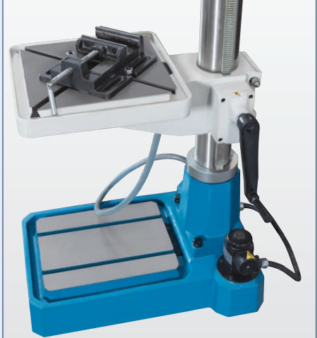
Coolant system is integrated in the machine base
