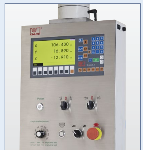
Swiveling control panel with integrated position indicator
