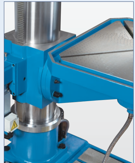
Large drill press table with circumferential coolant groove and ± 45° swivel range
