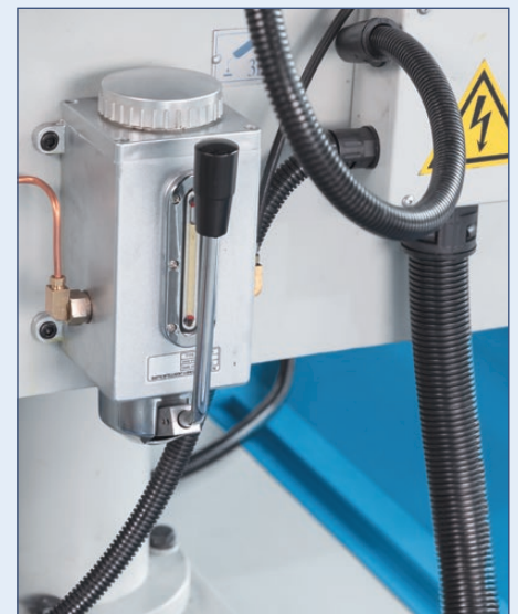
Central lubrication facilitates machine maintenance.
