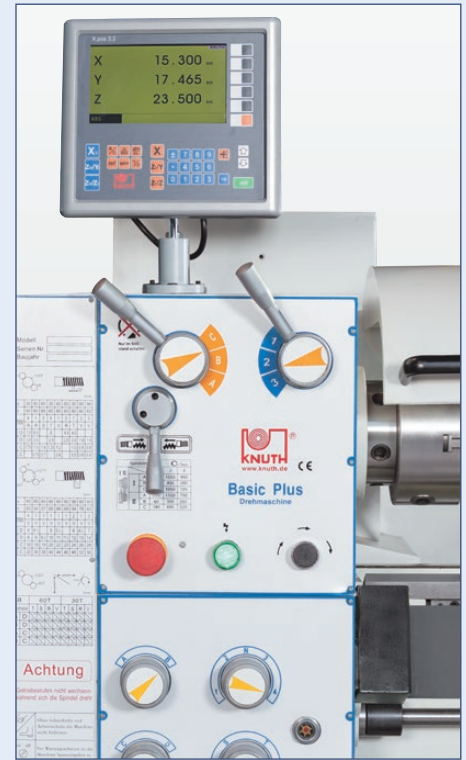
Positioning indicator on X, Z and Z1 axis
