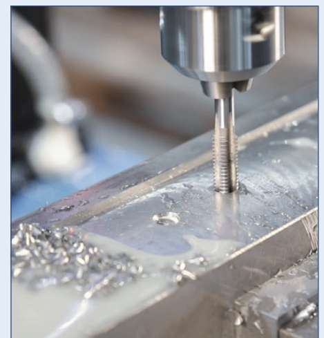
Tapping function is included in standard equipment
