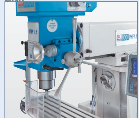
A hand-wheel for micro-adjustments allows precise quill positioning
