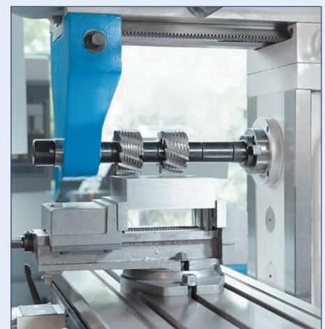
Horizontal spindle ensures efficient chip removal
