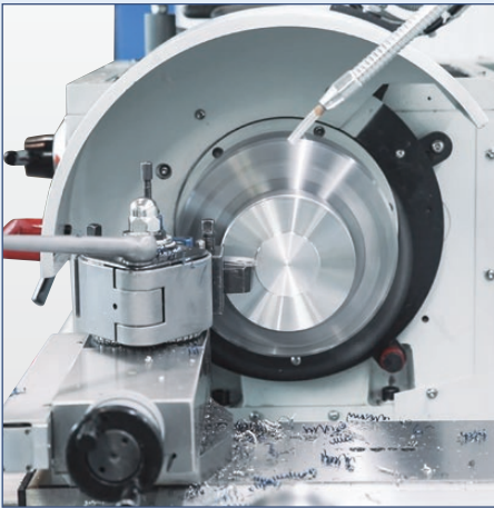
V-constant - during facing the spindle speed automatically adjusts according to the changing workpiece diameter
