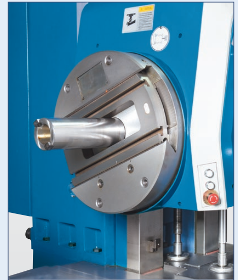
Facing slide with long stroke for internal turning
