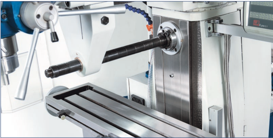
Solid top beam with outer arbor allows rigid mounting of long milling arbors
