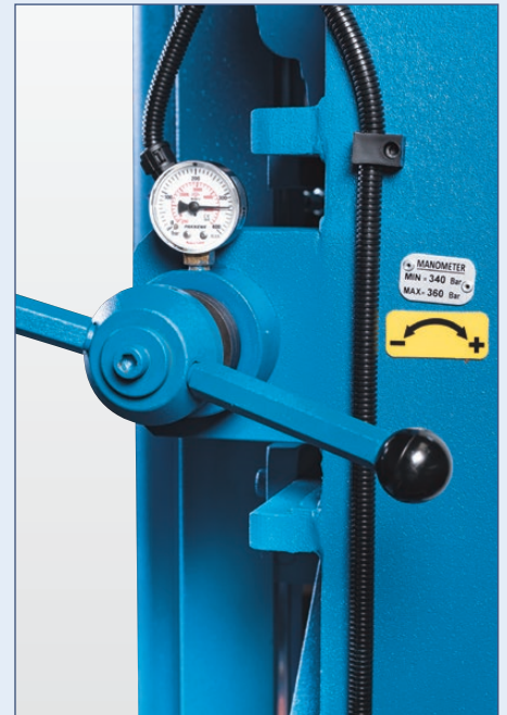
Pressure gauge ensures correct saw blade tension for increased blade life and cost reduction
