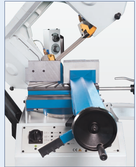
The manual vise on the SBS 235/255 features a quick-action clamping function
