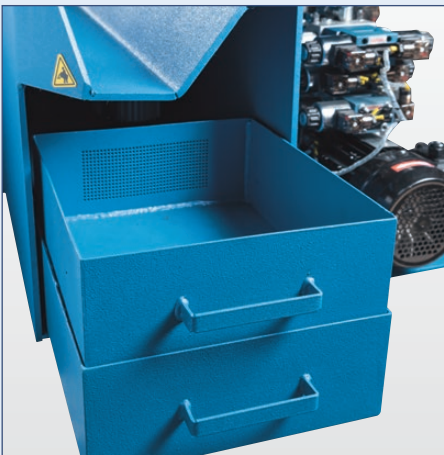
Removable coolant reservoir for simplified maintenance
