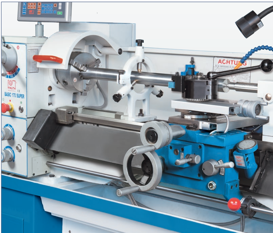
Long workpieces are supported in rigid rests
