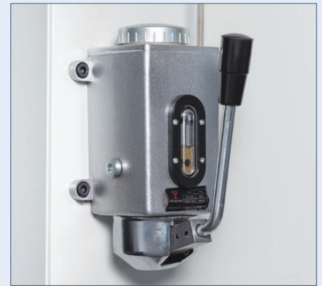
A central lubrication system ensures reliable lubrication of the column
