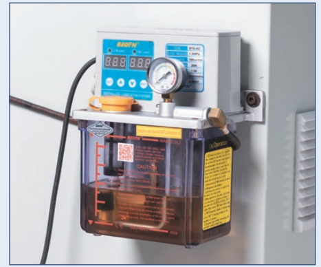
Continuous precision lubrication minimizes friction and wear of movable parts and increases the machine life
