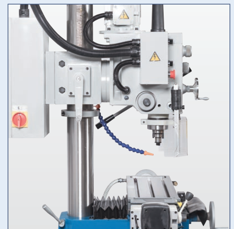
Gear head and table are vertically adjustable
