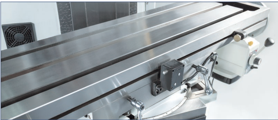
Cutter table swivels in X axis
