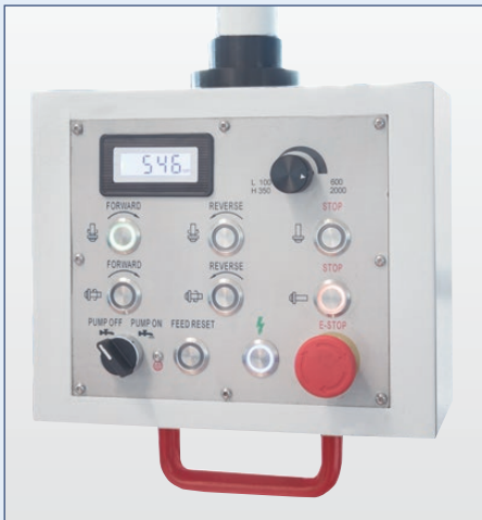
User-friendly intuitive control panel with speed indicator
