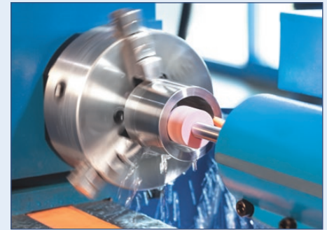
The maximum inside grinding diameter is 100 mm
