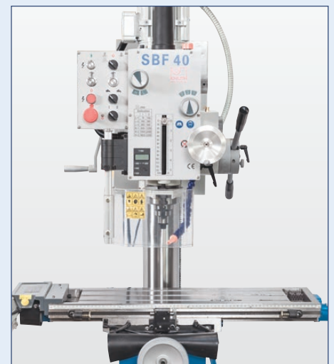
Gear head swivels to both sides
