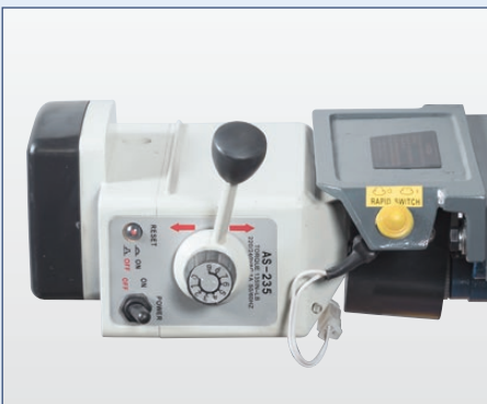
Infinitely variable milling table feed
