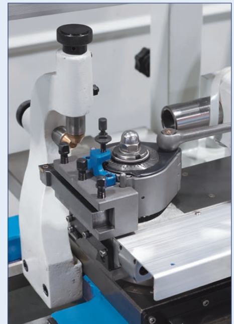
Quick-change tool holder system makes turning tools instantly available for use
