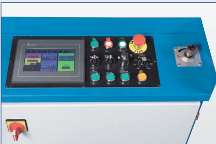
PLC control with touchscreen
