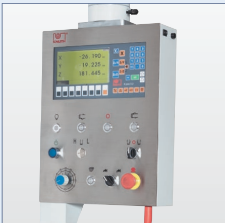
Control panel swivels for comfortable operation
