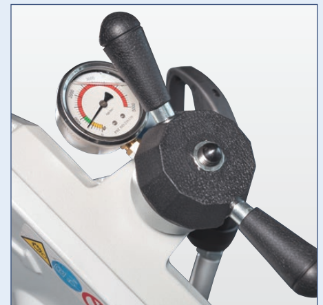
Pressure gauge for precise saw blade tensioning
