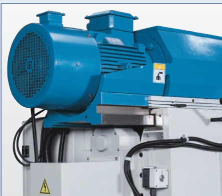
The complete drive is integrated in the heavy top beam that positions the cutter head
