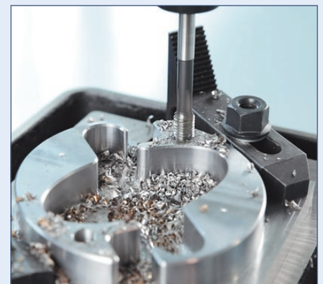
Thread cutting mode can be selected at the control panel
