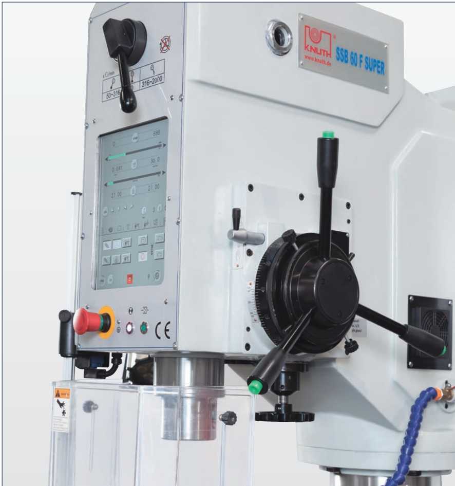
Electronically controlled servo quill feed with thread cutting function
