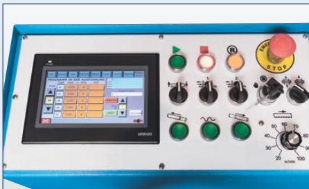
Reliable OMRON control with rugged touchscreen input panel
