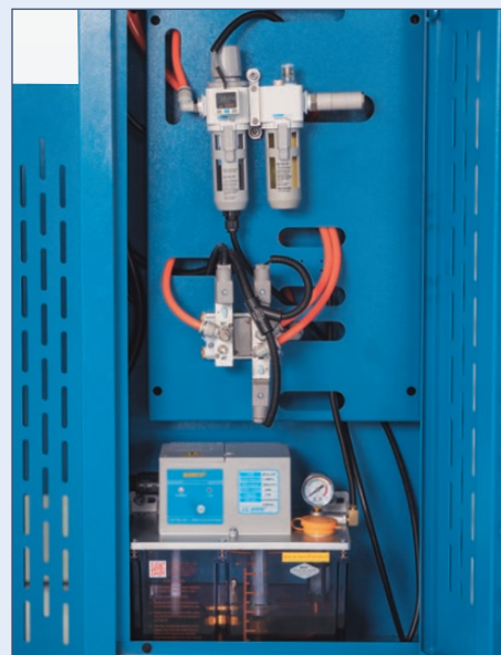
An automatic central lubrication system simplifies machine maintenance
