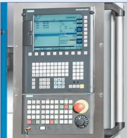
SINUMERIK 828 D – The powerhouse in the compact class of CNC controls
