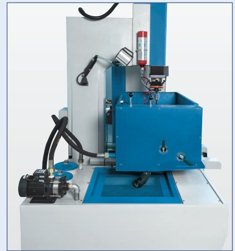
Large tank for dielectric mixture with integrated filter unit
