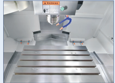
The guides in all axes are protected by robust stainless steel covers
