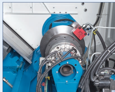
Spindle bore with up to 75 mm draw tube (Return 402M)
