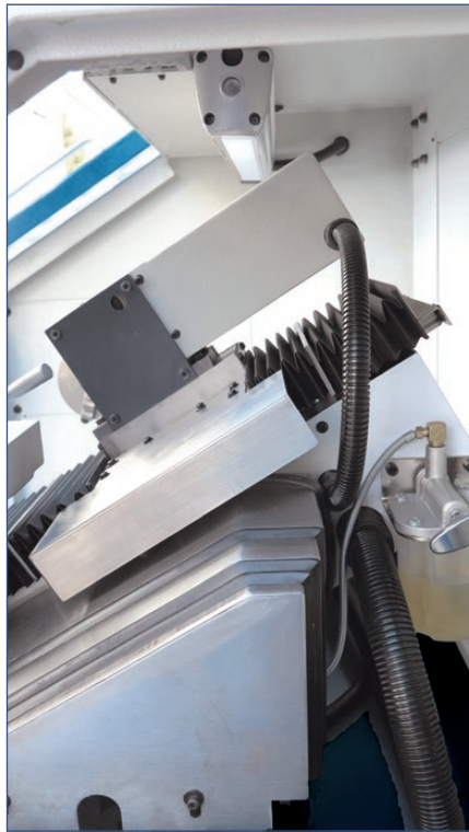
Inclined bed design optimizes work space and chip removal
