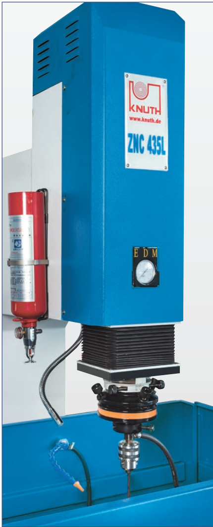
Fire extinguishing system for added safety
