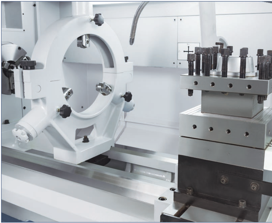
Heavy, automatic 4-station servo-driven tool changer for programmed tool changes
