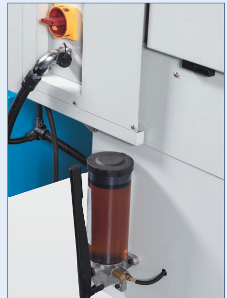
The central lubrication system simplifies maintenance
