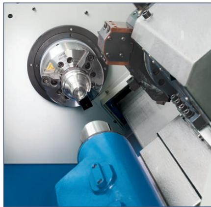
Rigid tailstock for exact workpiece alignment and support
