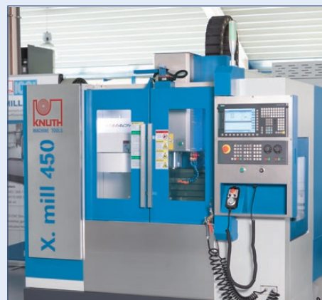
Work space is totally enclosed and can be equipped with an exhaust system
