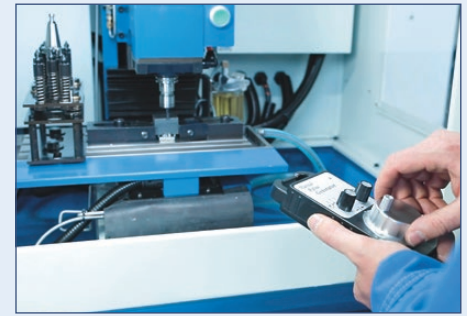
An electronic hand-wheel simplifies machine set-up
