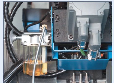
Manual central lubrication for reduced maintenance
