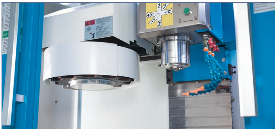
A 12-station tool changer provides for increased productivity, flexibility and safety during machining
