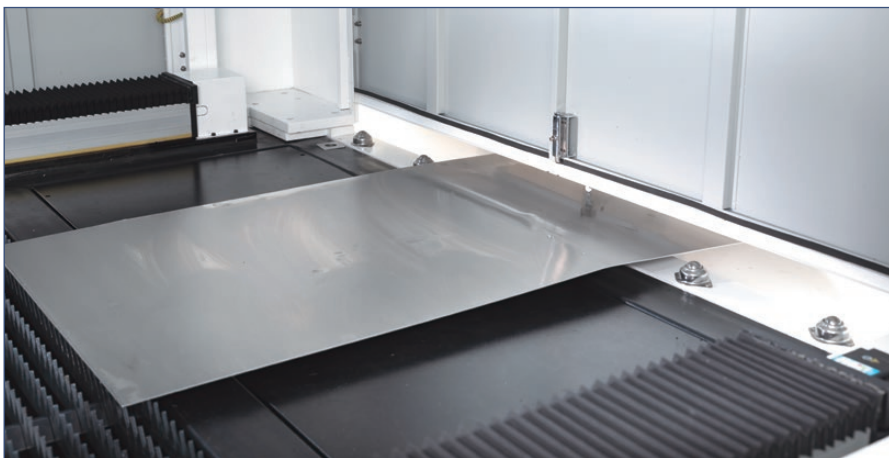
An enclosure pass-through allows feeding of small and medium-sized metal sheets
