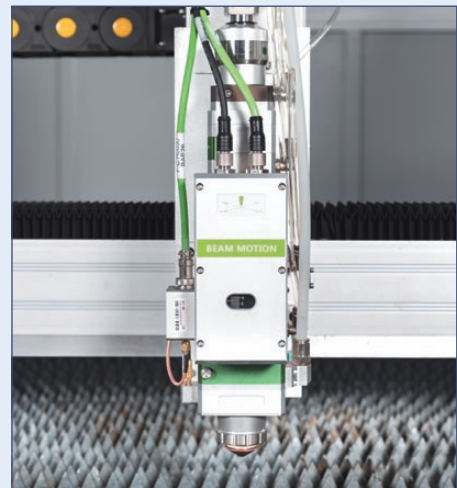
Cutter head with integrated collision guard, automatic focus positioning, and height control
