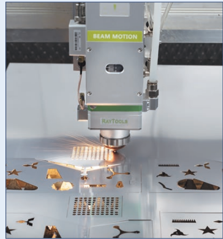
High-quality cutter head with Autofokus by RayTools
