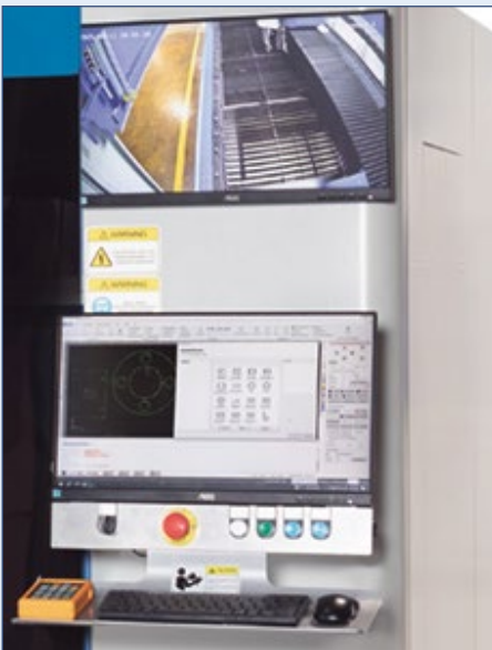
Complete system with CNC control (FSCUT4000)
