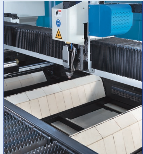
Fireclay plates protect the machine frame against thermal damages
