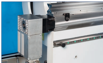
Motorized crowning included in standard equipment (optional for AHK V 13040 CNC)
