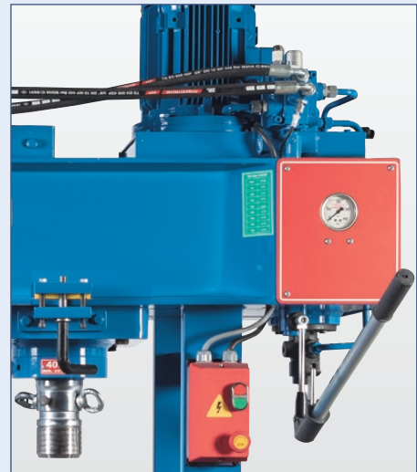
Manual operation allows for precise control of the press force. This is especially important when machining delicate contours, where precisely metered pressure is required
