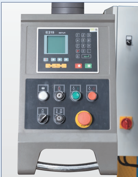
NC control for quick positioning of the back gauge
