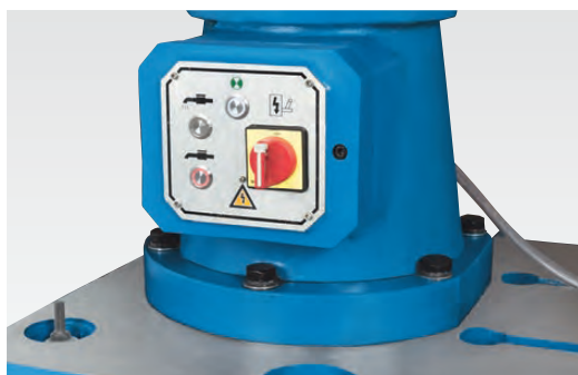
Rigid column base with central main switch
