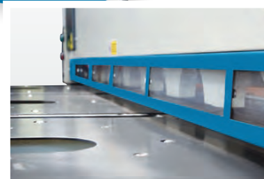
Material support rollers are recessed in the table for easy workpiece handling
