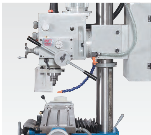
Automatic quill feed with 3-step gears
