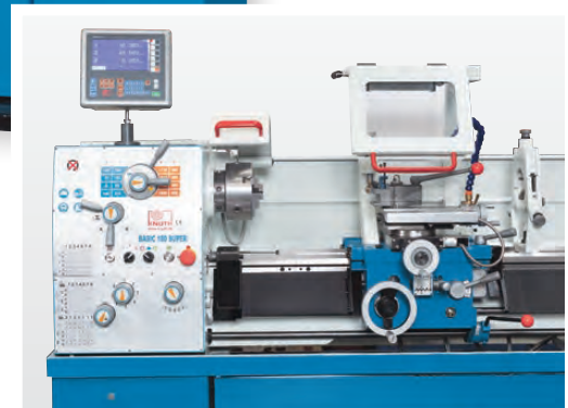
Select the optimum spindle speed for the Basic 180 Super via its 16-step main drive
