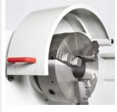
All models feature chuck guard with interlock system, spindle, spindle will stop if the guard is lifted during operation.
