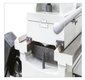
Possibility to offset the tailstock for taper turning.
