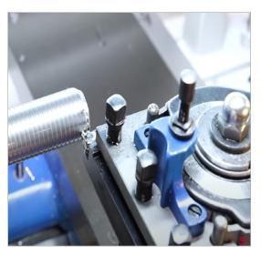
• This model is equipped as standard with quick type quick change tool post to easily switch the tools with repeat accuracy of 0,01 mm.
