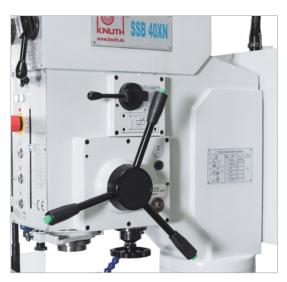
All buttons and levers are intuitive and clearly positioned, offering a convenient and ergonomic operation.
