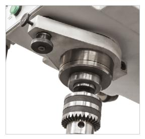
• The spindle is equipped with too disassembly and balancingdevice, which allow an easy tool removal and changing.
