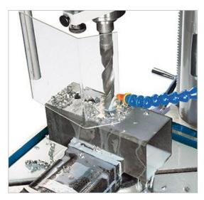
• The cooling system provides coolant to both the tool and the workpiece during machining. The flow rate of the coolant is adjusted by a ball valve.
