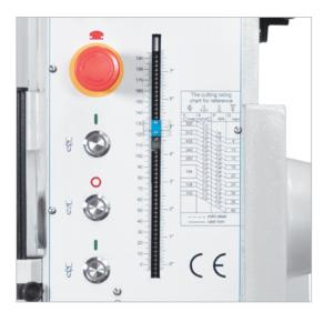
• The long quill travel can be manually adjusted using the depth stop. The automatic feed switches off when reaching the selected drilling depth.
