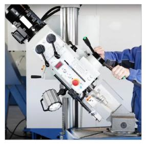
• The SSB 32 Xn model's tilting headstock makes it possible to drill angled holes in large workpieces that are mounted directly to the table.
