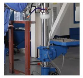
The table is equipped with a manual height adjustment mechanism and a rotating base, which allows it to be adjusted to the desired height and rotated to accommodate tall workpieces.
