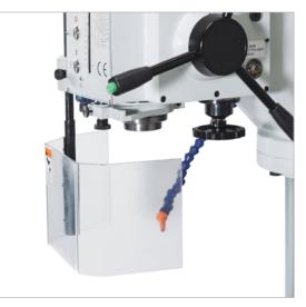
The height-adjustable spindle guard protects the operator from chips and coolant during operation.
