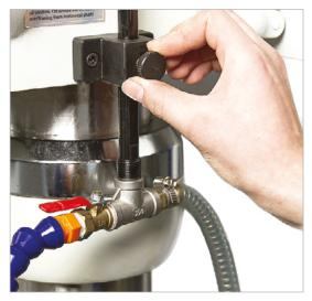
• Due to the movement of the headstock, the coolant system is outside the machine frame and its height can be easily adjusted.
