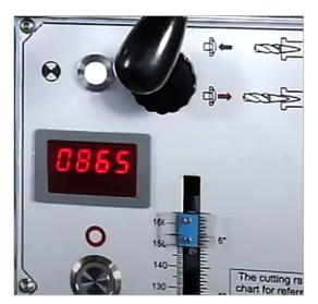
• This model features a digital display of the spindle speed, which allows the operator to easily monitor and adjust the speed of the drill bit.
