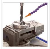
The coolant system is activated on the touchscreen, keeping the drill bit cool and preventing it from overheating.
