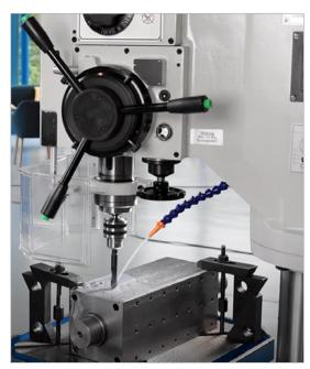
The built-in drilling assists system helps the operator in selecting the correct machining technology values, such as the spindle speed and feed, depending on the drill diameter and material.
