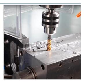
This series has integrated threading function. Once activated, the machine changes automatically the direction of rotation of the spindle when the selected depth is reached.
