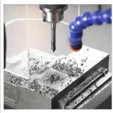
When the selected thread depth is reached, the machine automatically changes the dicrection of rotation of the main spindle.
