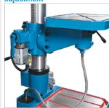
The height adjustment of the table is done by motor and is conveniently controlled from the control panel
