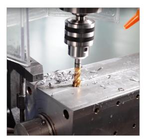
The tapping process is performed with automatic feed and the spindle speed is synchronized with the thread leads to ensures that the thread is done accurately.
