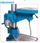
The height adjustment of the table is done by motor and is conveniently controlled from the control panel
