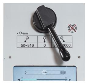
The spindle speed can be adjusted in two gear stages, providing a wide range of speeds for different materials and applications.
