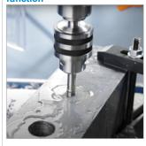
The tapping process is performed with automatic feed and the spindle speed is synchronized with the thread leads.
