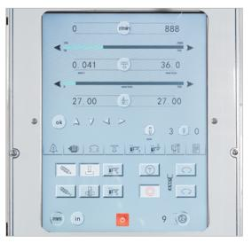
• Spindle adjustments are made through the wide touchscreen, which provides a convenient and intuitive way to control the machine.
