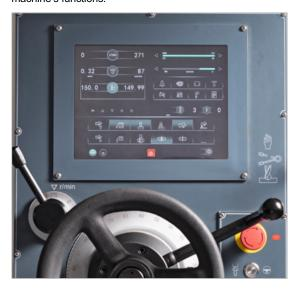
Drilling depth is electronically set, and the input value is checked by the system. On the screen the feed is displayed in two ways: feed per revolution and feed per minute.
