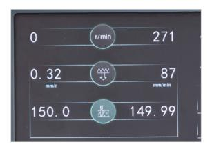
Measuring units for input and display can be selected by the operator (mm or inch).
