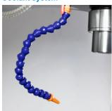
The high-performance coolant system is enabled at the touchscreen and will be turned on and off as a function of the main spindle
