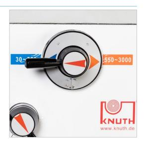
This series is equipped with an inverter, reducing the number of speeds to two, with infinitely variable speed adjustment
