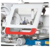
Large cover to protect the operator against chips and coolant splashes Fixed splash guard (wall)
