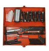
Tool box with tools for operating the lathe and maintenance
