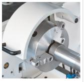
Chuck guard with integrated intelock system
