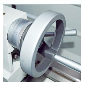
· The quill can be positioned with ease using a handwheel with precision scale
