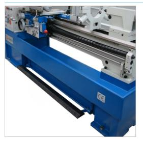
A heavy ribbed machine bed and a massive one-piece cast-iron frame provide the solid basis for this machine
