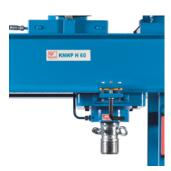
· Piston can be moved left-right to change the position of the pressing point.
