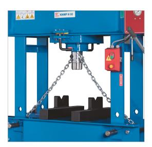
The heavy table can be easily adjusted to different heights with the help of the hydraulic cylinder, which is linked to the piston via a chain.
