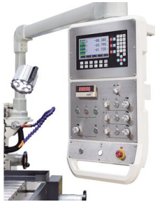
Feed rate and spindle speed can be switched and continuously adjusted at the control panel
