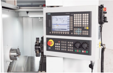
The tool turret can be fitted with tools for inside and outside machining
