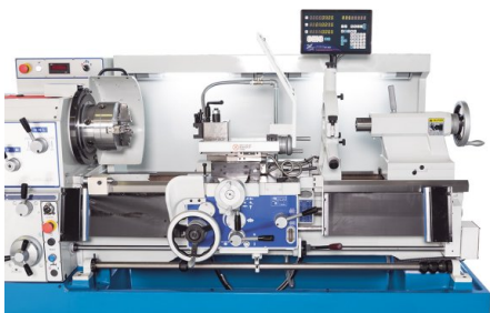
Adjustable stop cams automatically shut off the feed
