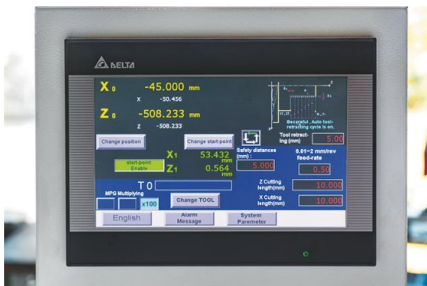
Large color touchscreen provides a graphic display of machining operations and lists editable parameters
