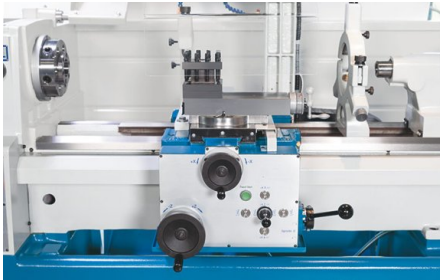
Axes are powered by high-quality servo drives that translate your hand movements with the precision and dynamics of modern CNC machines
