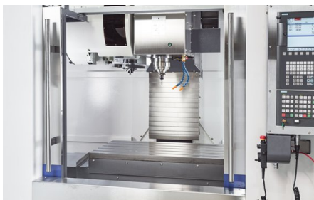
Rapid tool changing with dual-arm gripper
