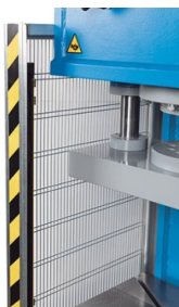
The workspace is protected by light curtains
