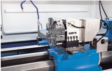
Automatic 8-station tool turret with hydraulic clamping
