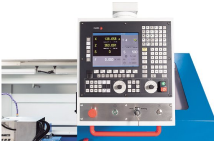
The Fagor 8055 CNC provides an intuitive workshop programming solution via simple graphic-based dialog buttons
