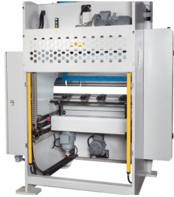
A large throat and narrow table ensure plenty of free space to accommodate complex bending
