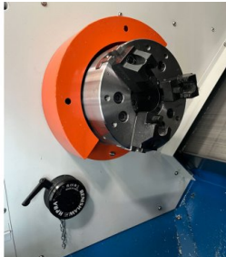
Quick-action clamping within the work space
