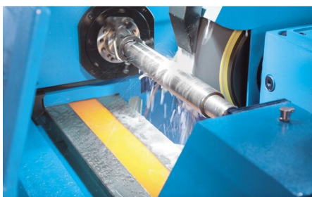
The hydraulic linear feed is infinitely variable and micro-adjustable
