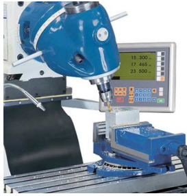
Cutter head swivels on 2 levels
