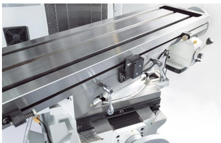
Cutter table swivels in X axis
