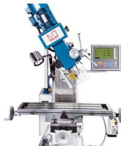
Swiveling cutter head with sliding quill
