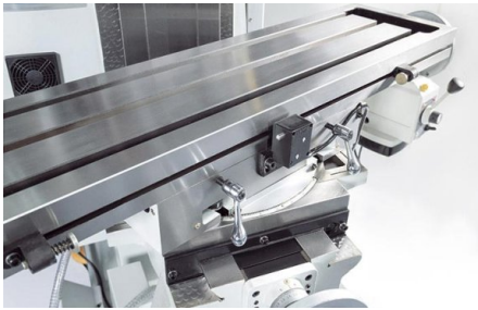
Cutter table swivels in X axis
