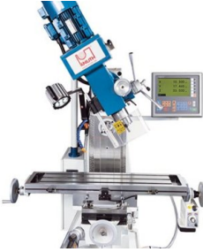
Swiveling cutter head with sliding quill
