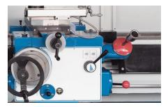
Support moves in linear and cross direction via motorized rapid feed for reduced down-
