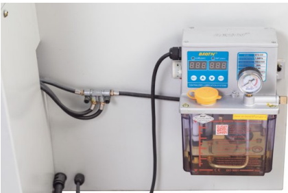
Continuous precision lubrication minimizes friction and wear of movable parts and increases the machine life
