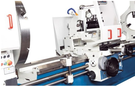
Rigid rests are included in the machine's standard equipment
