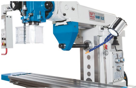
Precision-ground guideways with hardened surfaces for long-term accuracy and wear-resistance
