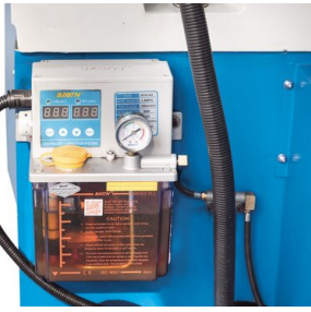
The centralised lubrication system reliably supplies all lubrication points with lubricant, making daily maintenance easier
