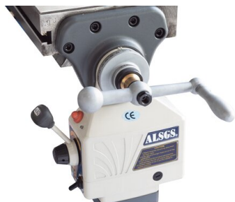
X and Y axis feature automatic and rapid feed modes
