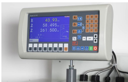
V-constant - during facing the spindle speed automatically adjusts according to the changing workpiece diameter
