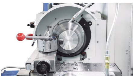
V-constant - during facing the spindle speed automatically adjusts according to the changing workpiece diameter
