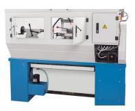
The work area is also accessible through large swinging doors on the back of the machine
