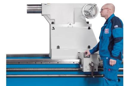
*Motorized positioning of tailstock (all models with a minimum center width of 3000 mm)*
