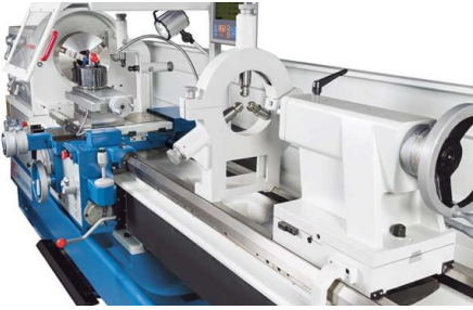
Rests ensure maximum precision when machining long workpieces
