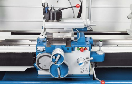
Support moves in linear and cross direction via rapid feed
