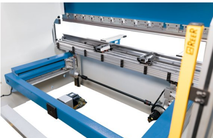
Option: Back gauge with controlled R axis
