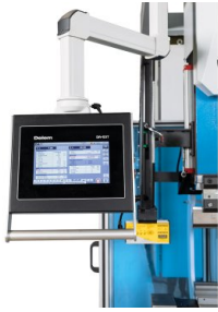
The compact DA-53T is a highly advanced touchscreen control solution for synchronized press brakes. The Delem touchscreen graphic user interface makes programming very easy.
