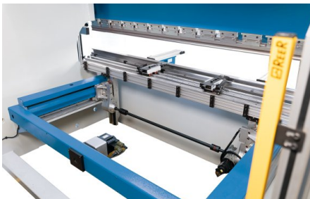
Option: Back gauge with controlled R axis
