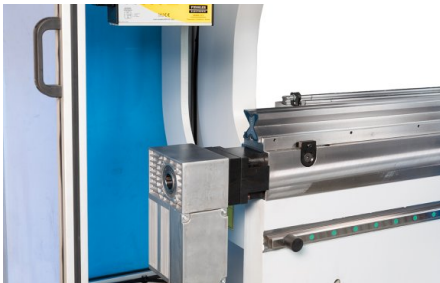
Motorized crowning included in standard equipment (optional for AHK V 13040)
