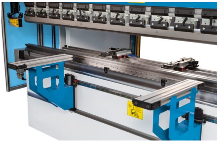
The rigid front support arms feature a ratchet mechanism for quick height adjustments
