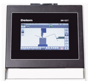
Machines are standard configured with 3 axis CNC controlled: Y1, Y2, X. Additional axes are available by request
