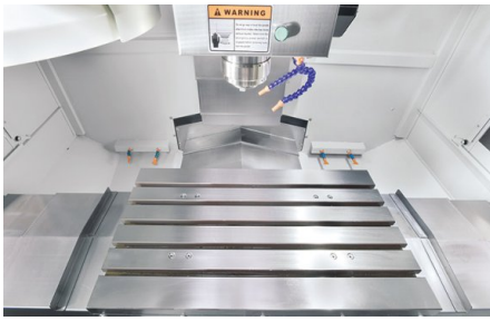
Solid machine table with 5 slots
