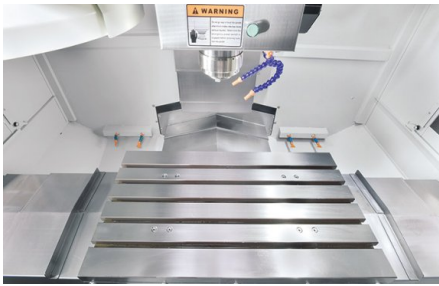
Solid machine table with 5 slots
