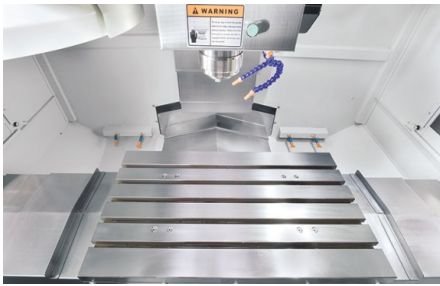
Solid machine table with 5 slots
