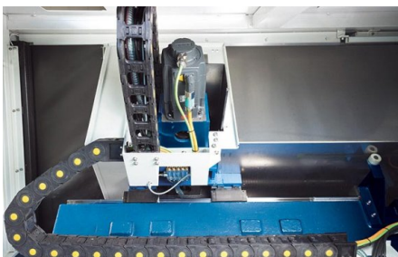
Siemens drive (here X-axis)
