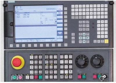
Siemens Sinumerik 828 D Basic for turning applications - a compact and user-friendly solution for lathes
