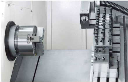
Linear tool changer with a driven tool
